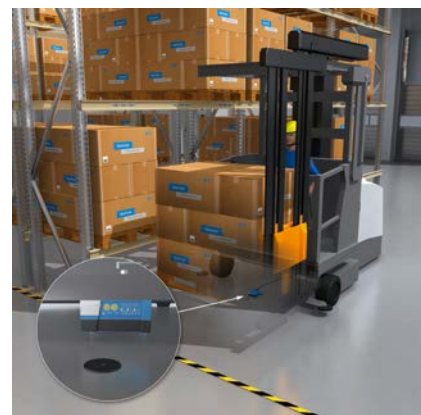
Driver assistance in a narrow aisle warehouse with RFID positioning
