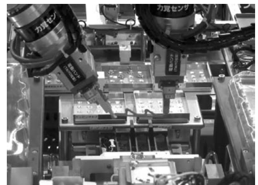
Enables installation work to be completed while gripper positions between robots are maintained.
