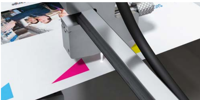
Detecting registration marks on printing machines.
